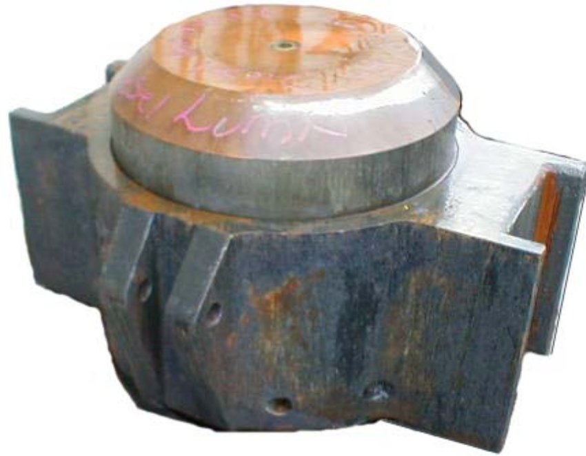
DCB Drive Cap Base 8 by 37 inch Weight without striker plate or cushion: 2,025 lbs
